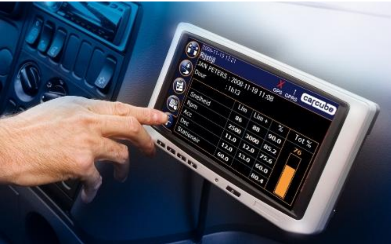
Figure 15: Board computer with CANbus interface displaying driving behaviour. Source: TTM (2010).
